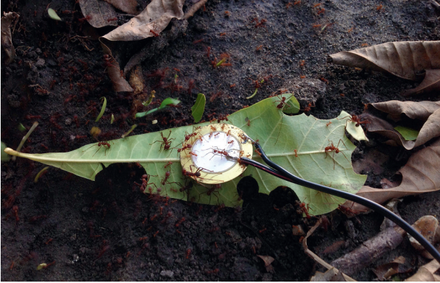
FIGURE 3 Photograph of the piezoelectric component which I usually employed in the field to record the stridulations of leaf-cutter ants. This image shows ants of the species Atta cephalotes cutting a leaf and interacting with the copper/ceramic disc near an entrance of their nest. The piezo is circuited into a low-cost amplifier in order to register acoustic vibrations.
